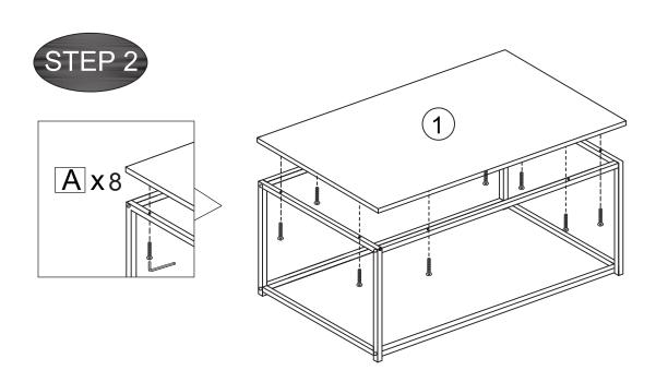
**STEP 4**: Lie the tabletop (1) on top of the assembled frame ensuring that the indents on the underside of the tabletop align with the openings on top of the assembled table frame.
