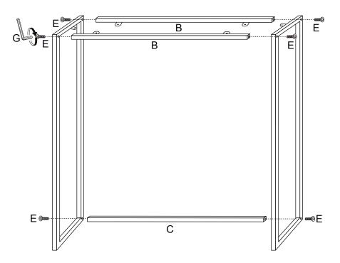
**STEP 2:** Insert the bottom fixing pole (C) into the leg frame as per image above and secure it into place with two fixing bolts and the allen key.
