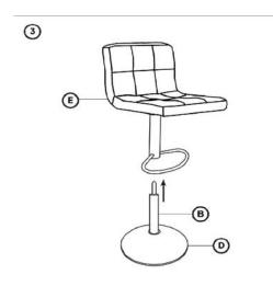
**STEP 5:** Slide the assembled seat and footrest on to the hydraulic stem until it cannot be pushed down any further.
