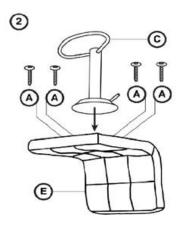
**STEP 3:** Using the Allan key (F), attach the footrest (C) to the seat using the four bolts (A) provided. Ensure that the seat and the footrest bar are facing in the same direction before securing into place. **STEP 4:** Carefully turn the stool upright and place on a flat surface, before fully tightening all bolts using the Allan key.
