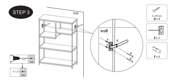
**STEP 3:** Insert the 4 wall plugs (F) into the pilot holes so that the wall plugs sit flush with the wall surface
