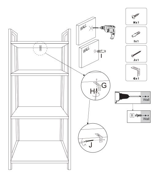
**STEP 3:** Insert the wall plug (I) into the pilot hole so that the wall plug sits flush with the wall surface.
