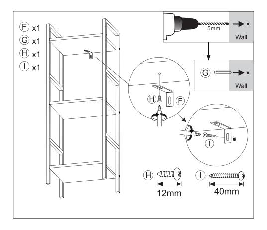
**STEP 3:** Insert the wall plug (G) into the pilot hole so that the wall plug sits flush with the wall surface.
